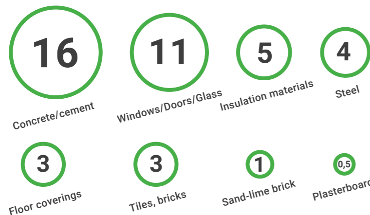
Fig. 13 | Greenhouse gas emissions from building materials in house construction in mn t of CO 2 e, source: dena (2022)
